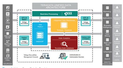
Figure 1. Voltage SecureData for Teradata
